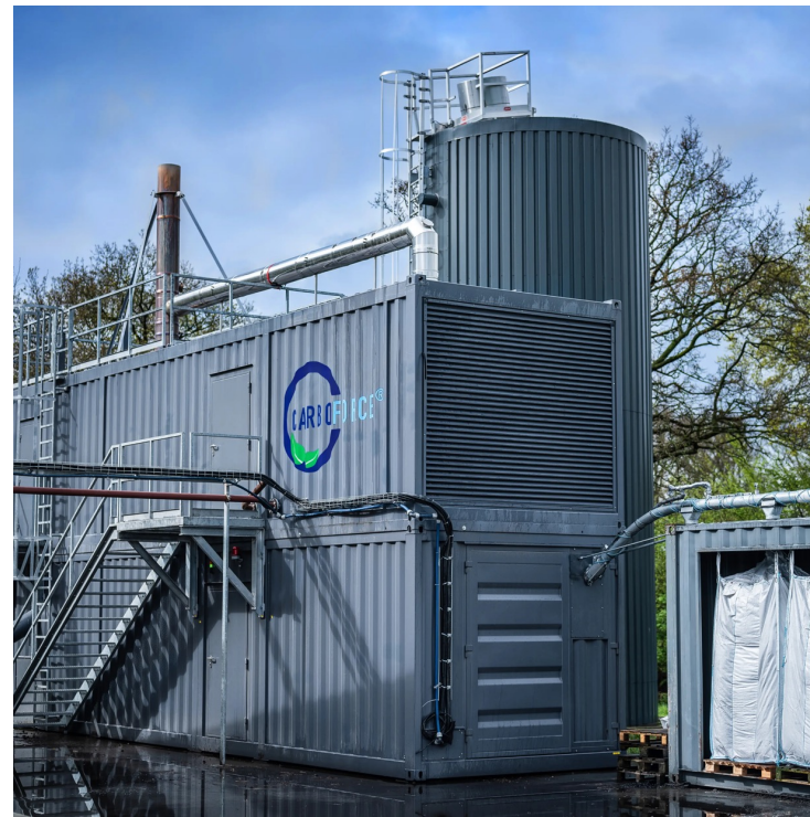
Containermodell (Biomasse 300 – 600 kg/h)
